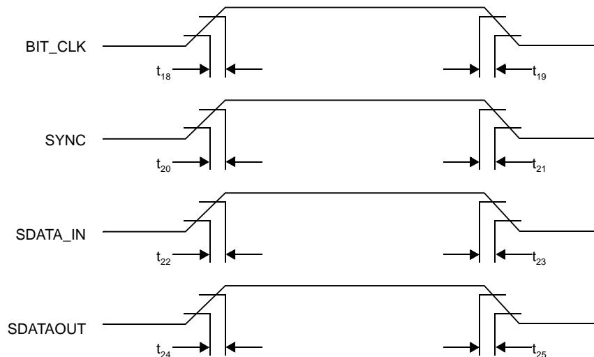
Figure 12 Signal Rise and Fall Times
