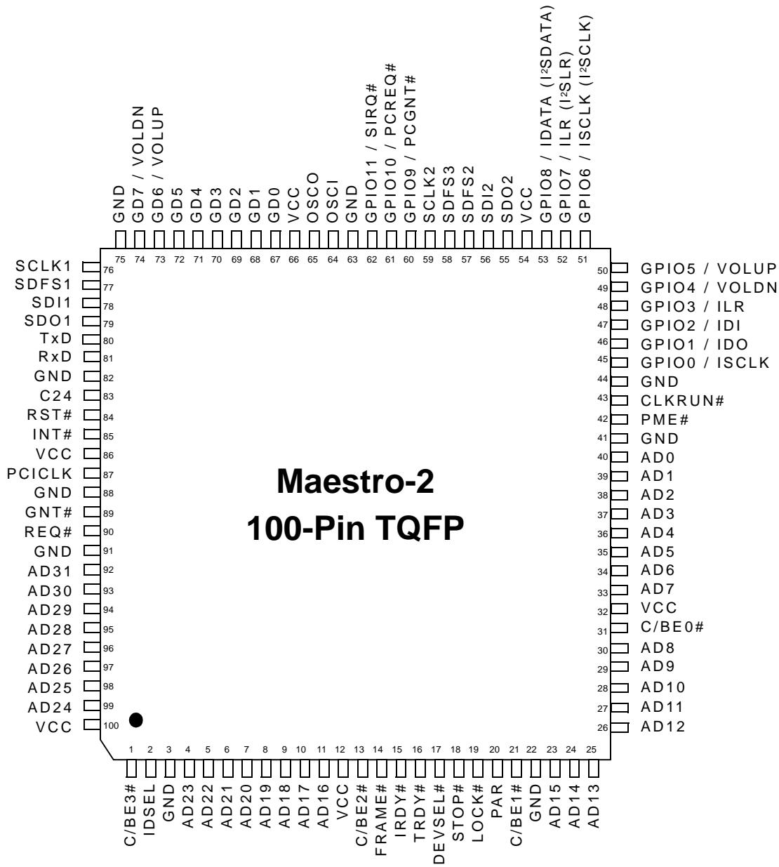
Figure 3 Maestro-2 Pinout
