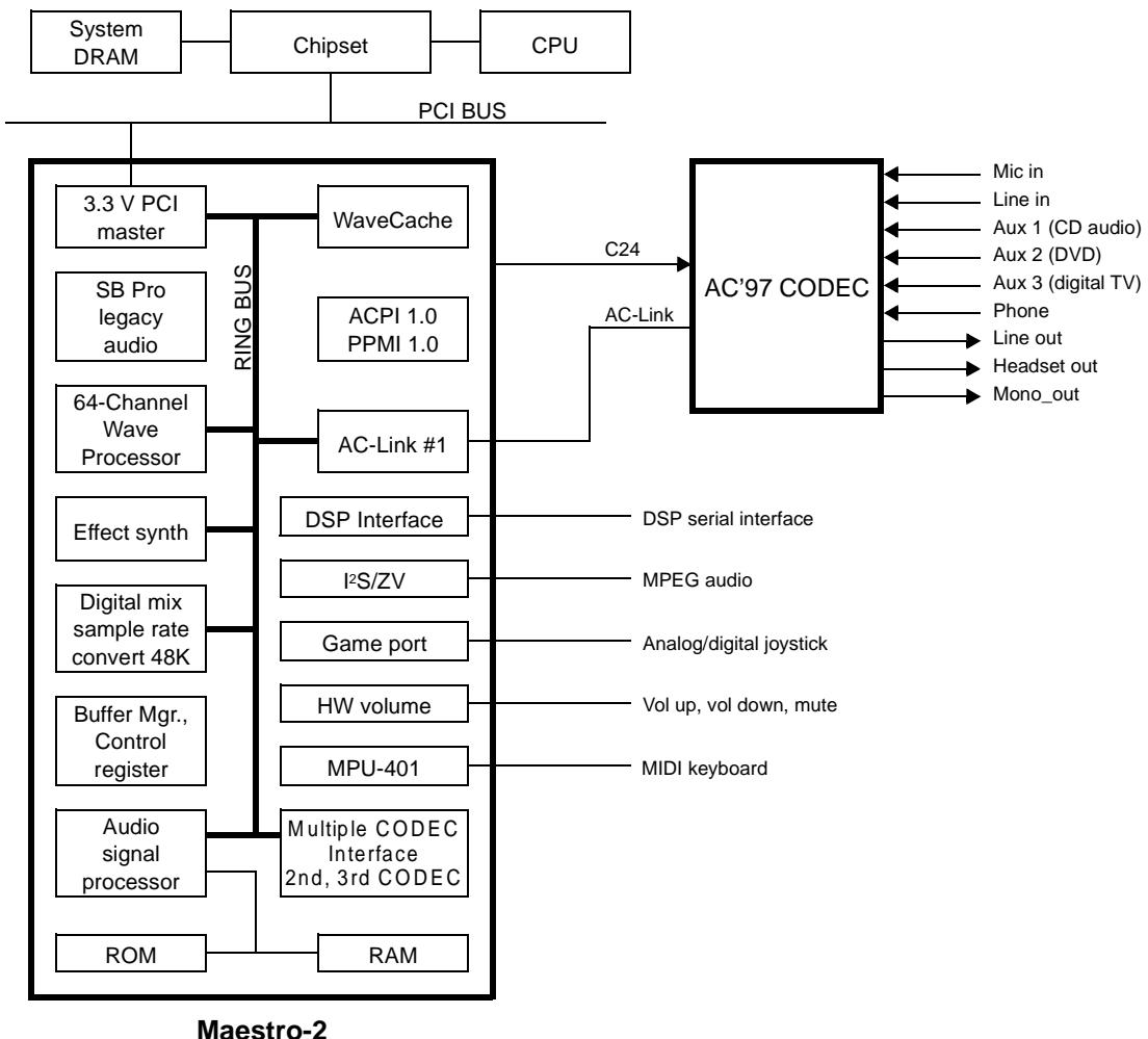
Figure 1 Maestro-2 Block Diagram
