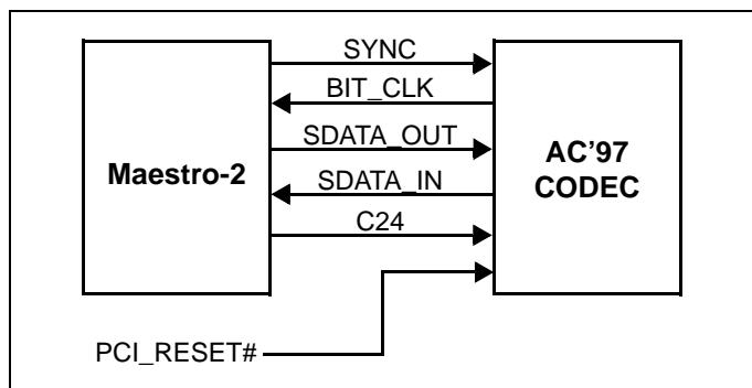
Figure 5 AC-Link Diagram
