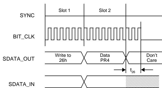
Figure 13 AC-Link Low Power Mode Timing
