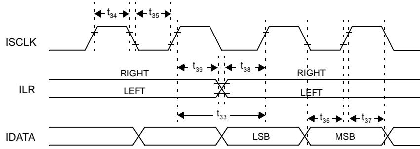
Figure 19 I<sup>2</sup>S Port Timing
