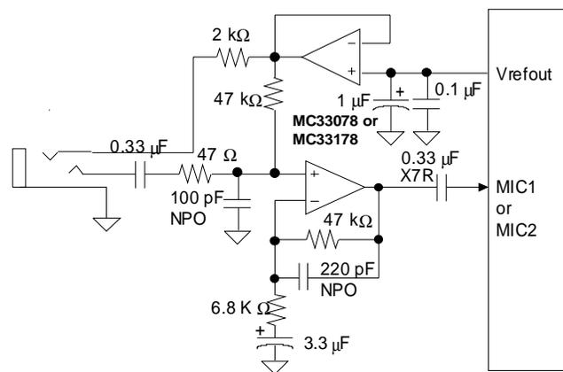
**Figure 6. Microphone Input**
