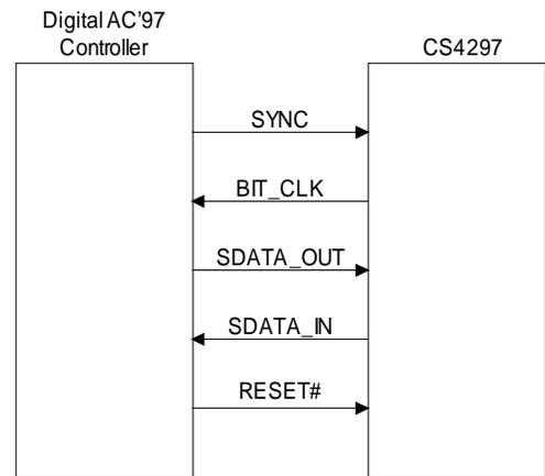
Figure 2. AC-link Connections
