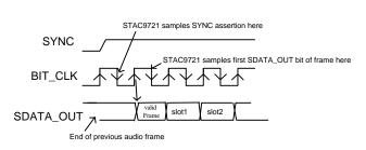
SDATA\_OUT's composite stream is MSB justified (MSB first) with all non-valid slots' bit positions stuffed with 0's by the AC'97 controller.
