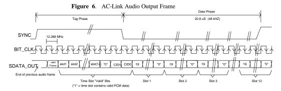
A new audio output frame begins with a low to high transition of SYNC. SYNC is synchronous to the rising edge of BIT\_CLK. On the immediately following falling edge of BIT\_CLK, the STAC9721/23 samples the assertion of SYNC. This following edge marks the time when both sides of AC-Link are
