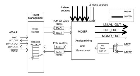
Figure 2. STAC9721/23 Block Diagram
