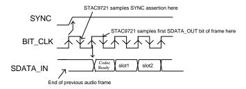
SDATA\_IN's composite stream is MSB justified (MSB first) with all non-valid bit positions (for assigned and/or unassigned time slots) stuffed with 0's by STAC9721/23. SDATA\_IN data is sampled on the falling edges of BIT\_CLK.
